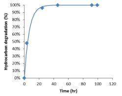
This figure shows the complete hydrocarbon degradation in TPH contaminated water using FBB technology.
