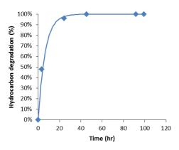
This figure shows the complete hydrocarbon degradation in TPH contaminated water using FBB technology.
